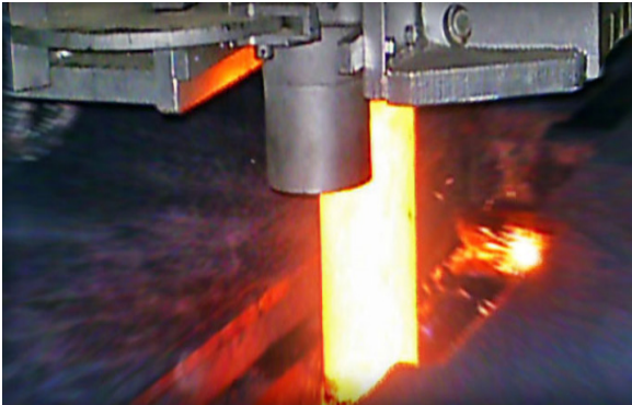
Fig. 1. Submerged entry nozzle in continuous casting
